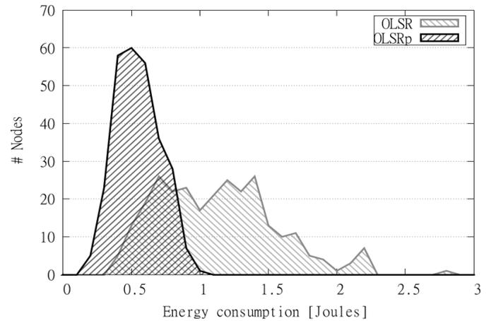
Figure 5. Histogram of energy consumption by number of network nodes
