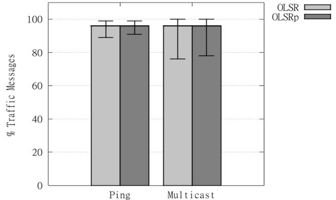
Figure 8. Comparative traffic produced by ping and multicast messages
