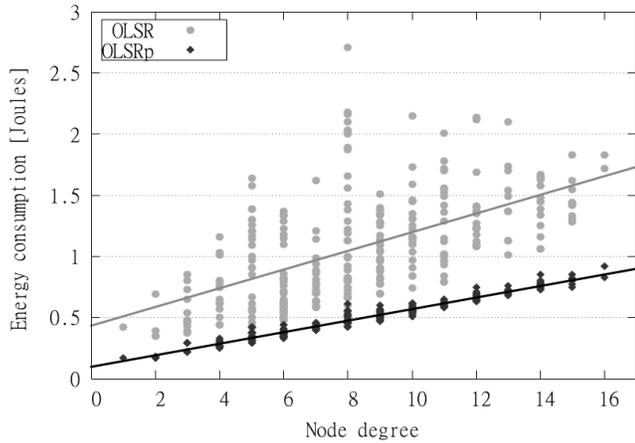
Figure 6. Relationship between node degree and energy consumption
