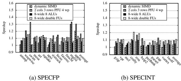
Figure 12: Comparison with SIMD and 8-way out-of-order
